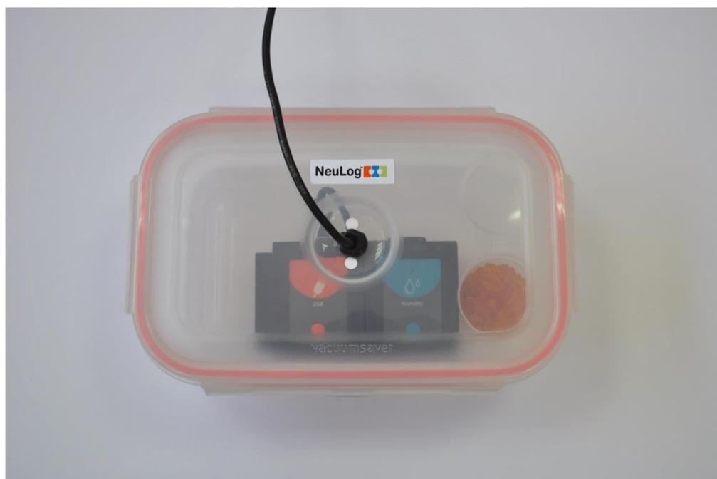
2. Make sure you have a sample container with 12 g of silica gel (around 4 teaspoons). Before you start the experiment, keep the container closed.
